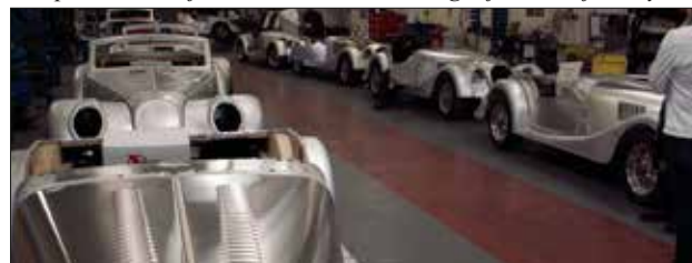
A batch of bare, unpainted steel-chassis 4/4s ready for fitting of small parts
