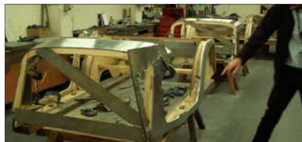
Aluminium panels fitted to ash frames. Every part and even complete bodies for a rebuild can be bought from the factory
