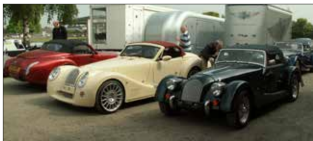
The two main types of Morgan, newly-built. Two modern models on left, built on alloy monocoque base unit. On right is traditional leaf-sprung 4/4, built on steel chassis. Production of the latter began in 1936 and continues to this day, making it the world's longest-produced car of all time.
